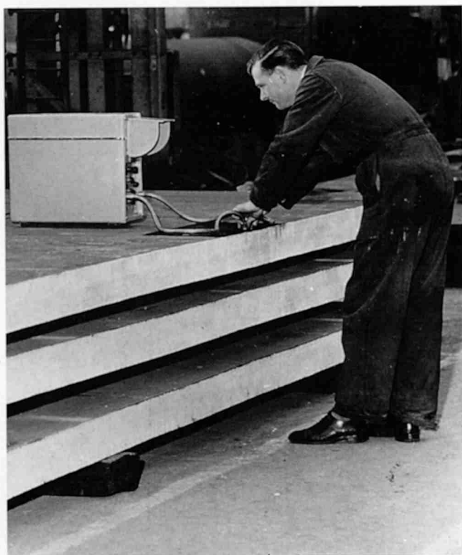
Fig. 1.5 A KH Mk4 flaw detector, c. 1956 being used by Mr Jim Davis in the Babcock and Wilcocks factory to test steel plates. Soon after his first meeting with Professor Ian Donald, Tom Brown arranged the loan of an instrument of this type from KH to replace the Mk2 (Fig. 1.4). The Mk4 was used for most of the early A-scan experiments and then became part of the contact B-scan machine in Fig. 1.6.
